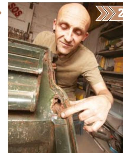
**2** Door pillar/shut: this area isn't available as a repair section, so will have to be fabricated. This area is triple-layered for strength, so unless the rot is fully cut out and the metal replaced, any rust will be trapped.
